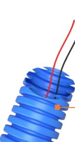
Protection pipe is made from polypropylene (PP). Outside diameter is 16 mm and inside diameter is 11.1 mm with compression strength 750 N/5cm.
